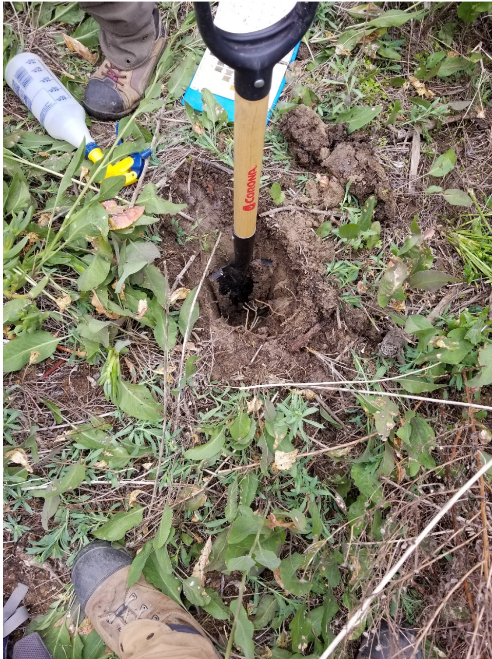
Photo 6 - View looking at Soil Test Pit No. 3; low chroma soils, redox features, and wetland the presence of wetland vegetation. The lack if wetland hydrology indicators did not meet the criteria for federally jurisdictional wetlands but do meet the criteria for jurisdictional wetlands by the CCC.
