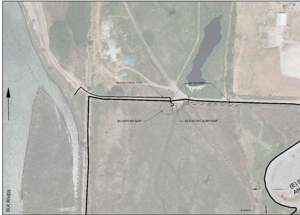
Figure 15. Area 1 dewatering schematic showing planned dewatering set up near Pound Road.
