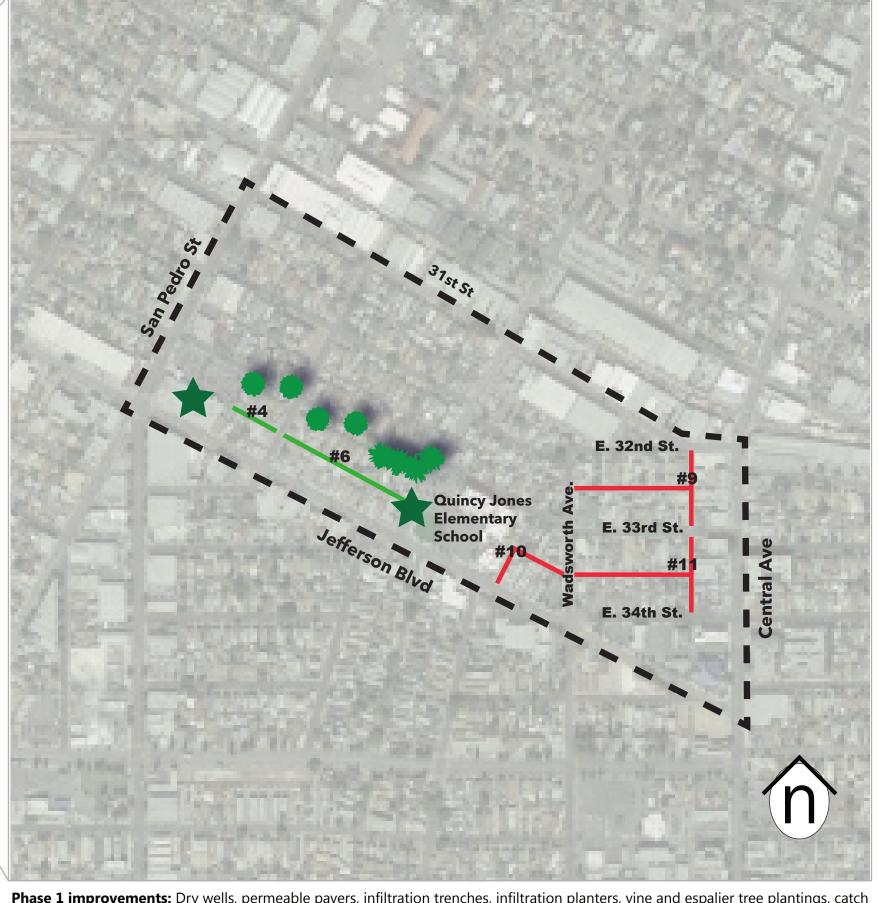
**Phase 1 improvements:** Dry wells, permeable pavers, infiltration trenches, infiltration planters, vine and espalier tree plantings, catch basins with trash inceptors, street trees, trash receptacles, dog waste bag dispensers, water quality monitoring equipment, mural art, interpretive signage and funder acknowledgment.
