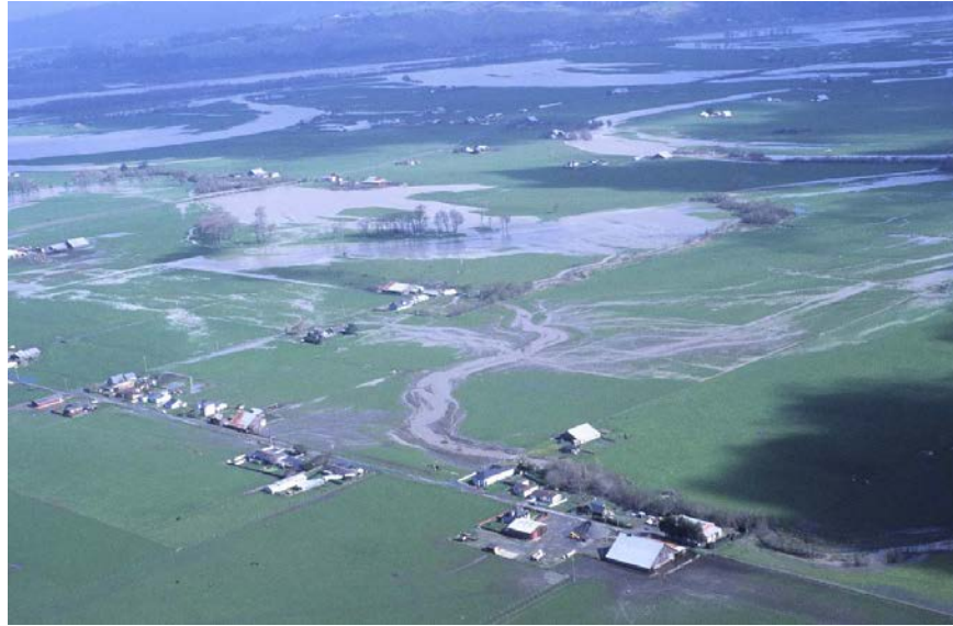
PHOTO - Flooding at lower Williams Creek. Salt River historic channel is in mid-ground with scattered trees along channel. A sediment plug in this location blocks the flow of 42% of the watershed, causing chronic flooding and ponding and reducing sediment transport capacity.
